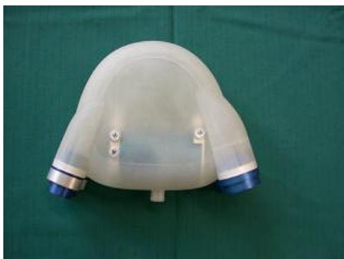
Fig. 1 The DLR-Heart, a Left Ventricular Assist Device
