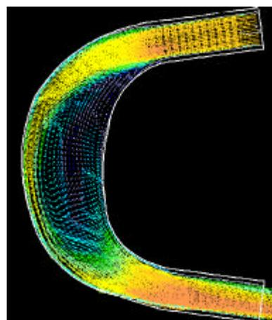
Fig. 6 Flow field, measured with PIV
